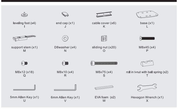
**IMPORTANT:** Ensure that you have received all parts according to the component checklist prior to installation. If any parts are missing or faulty, contact your place of purchase for a replacement.
